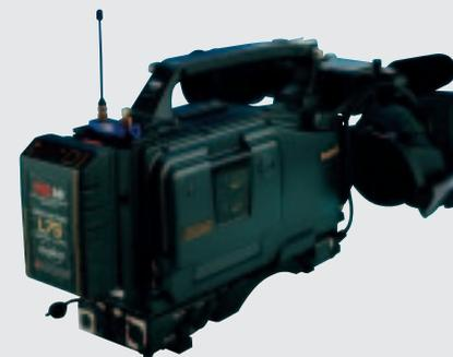
The CXiR slots into the latest professional digital ENG camcorders including those from Ikegami, Panasonic, Philips and Sony. If your camera doesn't have a dedicated receiver slot, you can use the CXiR externally by employing the six pin Lemo™ adaptor, with an appropriate custom designed bracket to mount the receiver.
