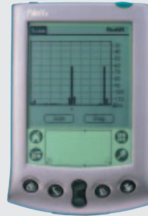
The **Scan** function on the pull down menu takes the guesswork out of finding a free channel in your location. The AudiR application allows the user to scan all 32 frequencies in the CXiR receiver, giving the user a bar-graph display of the scan, indicating the RF signal levels in dBm. The scan function effectively gives the sound mixer a dedicated handheld spectrum analyser.
