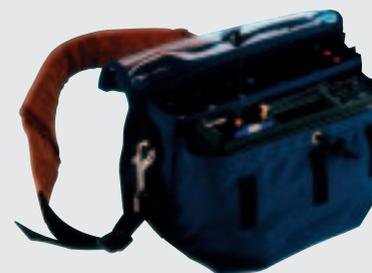
The CXiR fits easily into a typical documentary bag. A two-channel rack, which incorporates a slot for NP1 battery is also available.
